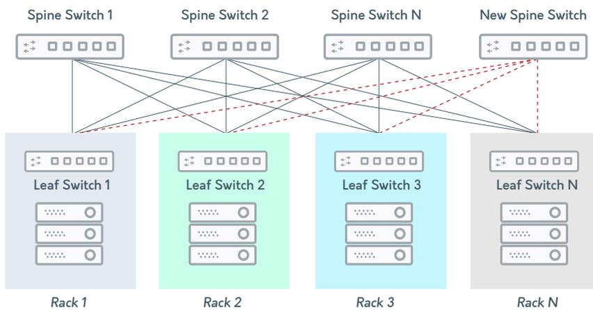
When a new Spine Switch is added, it requires the addition of a new physical connection to each existing leaf switch.
