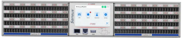
Figure 3a: Port Mapping: Duplex LC (Front view)
